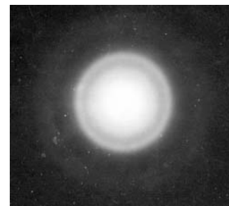
Fig. 5 SAED pattern of the as-formed SiCN
